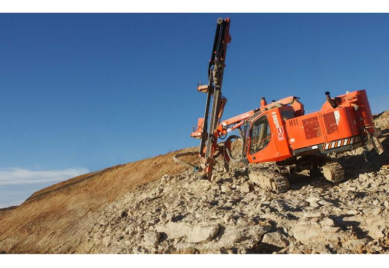
Sandvik DX800 is a hydraulic, self-propelled, self-contained, crawler based surface drilling rig equipped with a cabin (F.O.P.S. and R.O.P.S.) and rod handling system.
