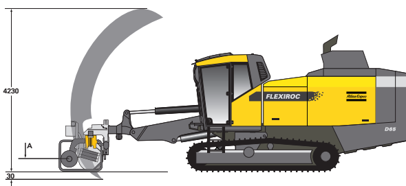
Toe-hole drilling reach for short feed
